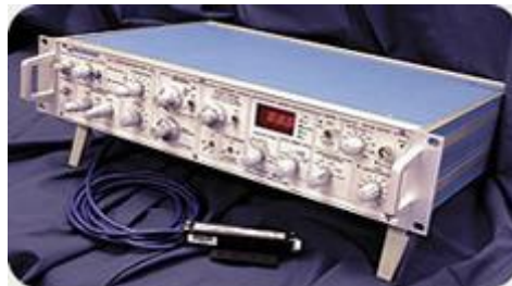
Figure 30: Axon™ Axopatch™ 200B microelectrode Amplifier
